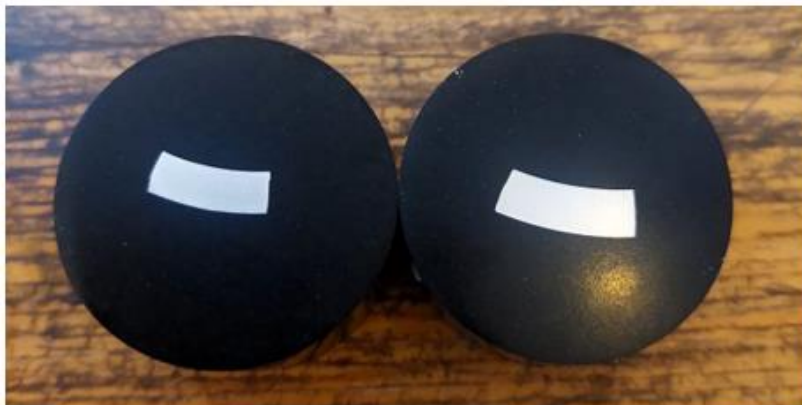
Gambar 4 Proses Mounting Sampel
