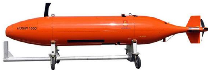
Figure 24 AUV with Multibeam Echosounder, Subbottom Profile, Side Scan Sonar
